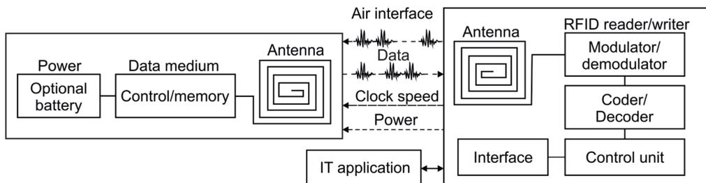
Figure 3. The working principle of RFID
